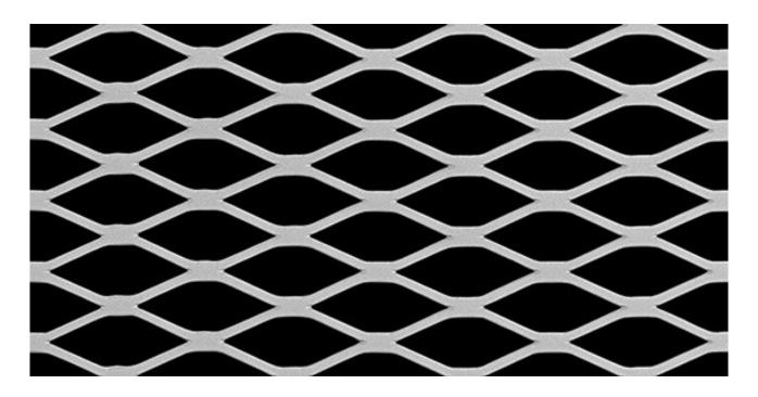
LW Aperture:33.53mmStrand Width:2.31mmSW Aperture:12.45mmThickness:1.14mmWeight:0.87 kg / m2Open Area:73%
